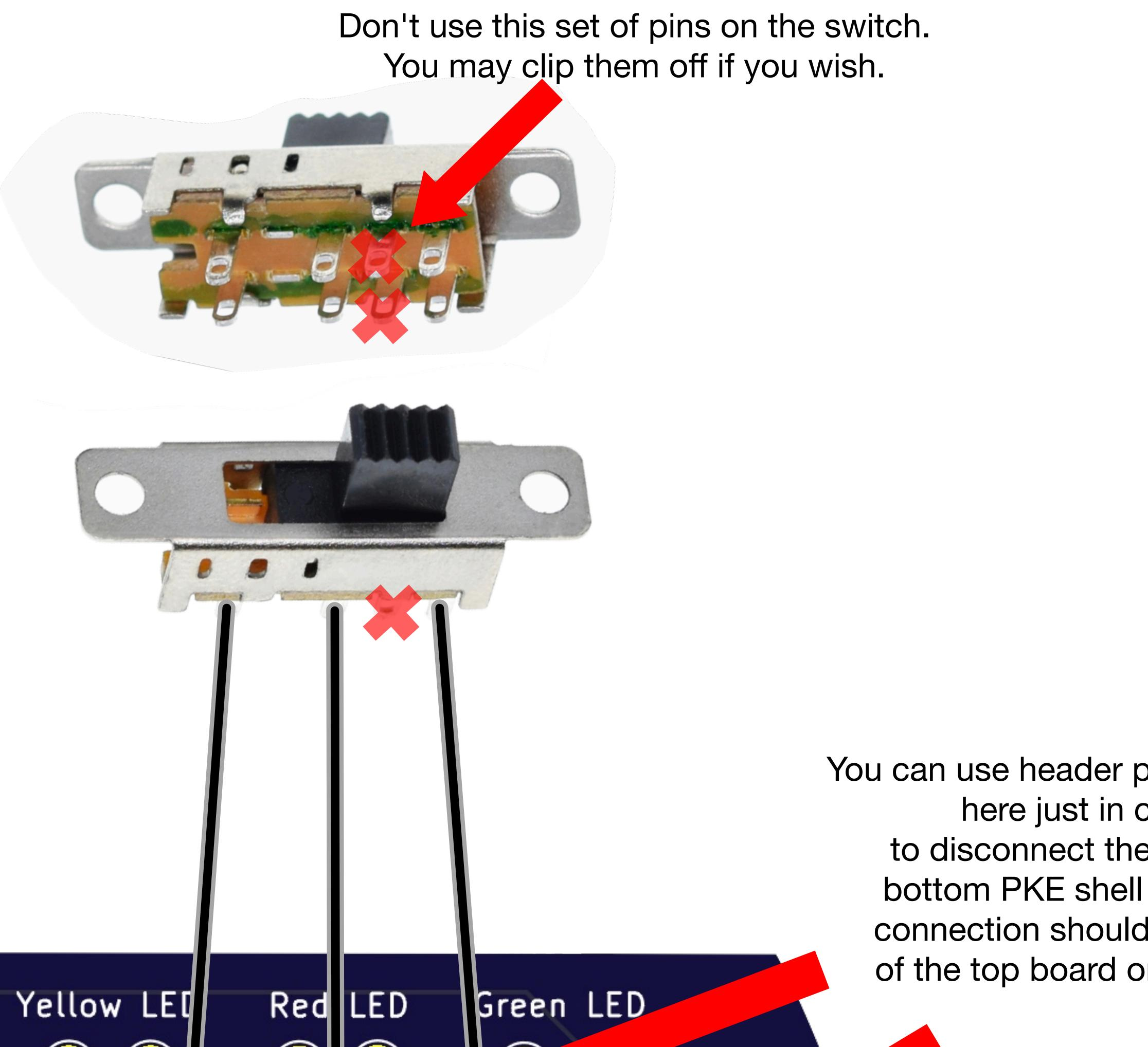
You can use header pins and DuPont connectors here just in case you ever need to disconnect the top PKE shell from the bottom PKE shell for maintenance. These connection should be made on the bottom of the top board on the side facing inward.
