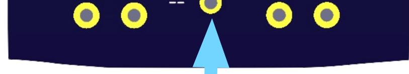
You can use 7 or 8 pins here. The last pin is just in case you can't find 7 pin connectors should you choose to try those types of connections. If you don't want to use a header pin, you can just solder the wires directly to the board.
