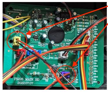
Unplug the yellow power connector from the Haslab circuit board.
