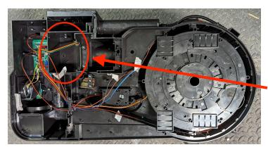
Make sure there are no wires obstructing the installation of the Talentcell into the pack.
