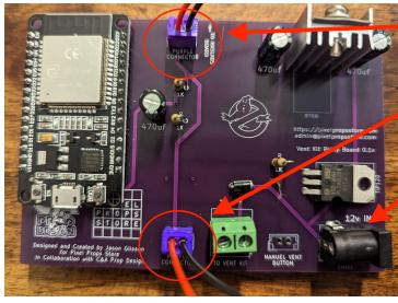
Connect the other end of the purple JST connector to the purple connector on the Haslab Relay Board.
