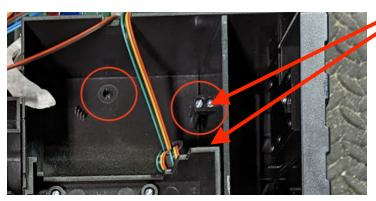
Remove the two screws holding the side panel in this area and remove the side panel.
