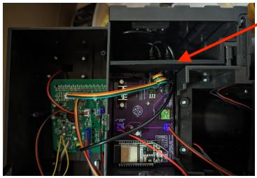
Install the provided side panel with the cables going under it so they are reachable from the power cell box.
