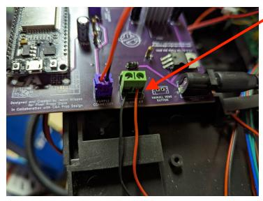
Connect the vent kit wires to the terminal connector labeled "To Vent Kit".
