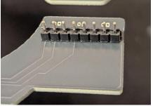
4. Slide the accelerometer onto the pins and solder the pins to secure the accelerometer. Only the first four are used so you can solder just those four.
