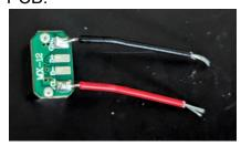
8. Next solder the assembled USB-C PCB and wires on to the main PCB board
