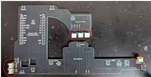
2. Attach the soundboard by aligning the surface mount pads on the soundboard to the pads on the PCB. Make sure there is no gap between the PCB and the soundboard. Assure there is enough solder joining the pads to the soundboard. The soundboard orientation must match the picture.
