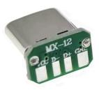
7. Solder one wire to the GND on the USB-C PCB and the other wire to the VCC on the USB-C PCB.
