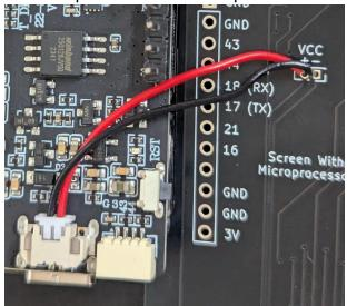
17. Connect the USB-C PCB to the microprocessor and screen
