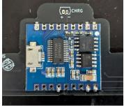
3. Next, connect the accelerometer. Feed the provided header pins through the back of the PCB.
