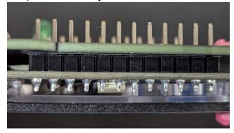
19. Solder all pins for the microprocessor and use wire cutters to remove the remaining pin lengths as close to the PCB as you can.
