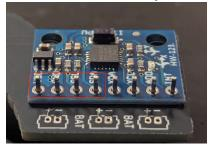
5. Snip the remaining length of the pins off flush with the accelerometer on the top and the bottom then solder
