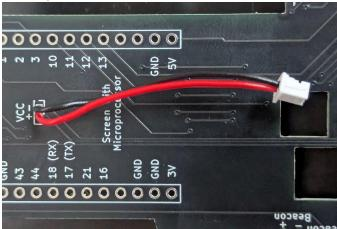
16. Connect the wire connector to the back of the microprocessor and screen being careful not to bend the wires inside the female connector.
