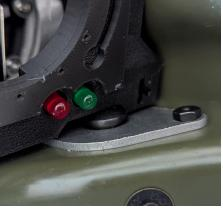
5. Once the insert is dropped in, line the side holes on the insert up with the side knob screw holes in the internal aluminum plate. Some slight pressure may be needed to line these side knob holes up.
