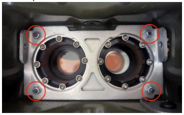
4. Drop the assembled kit into the goggles at an angle so you are avoiding the external battery screw.
