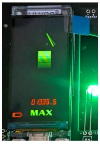
22. Test all movements of the kit and make sure the bar graph animations work correctly as well as the sound. You should be able to pivot the PCB up or down at around 45 degrees to trigger the sound change and the bargraph to green.
