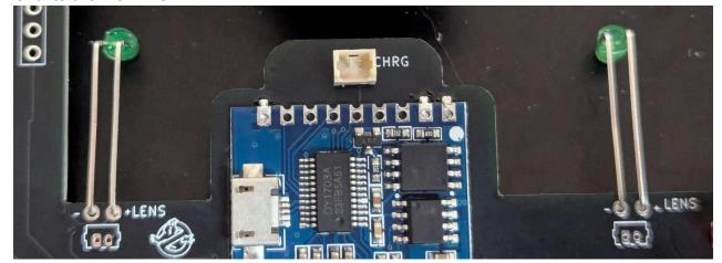
15. Cut the remaining connector wire that you used earlier about 2 inches long and solder into the VCC spot on the main PCB.
