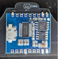
3. Next, connect the accelerometer. Feed the provided header pins through the back of the PCB.
