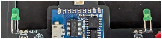
14. Once they are bent at 90 degrees, bend the entire LED and lead up 90 degrees so that it sits level to the main PCB.
