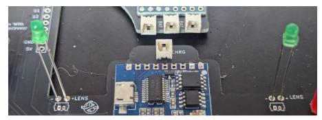
13. Once the LEDs are soldered into place, use a pair of needle nose pliers to bend the top of the LEDs to 90 degrees starting at the two lead marks towards the top.
